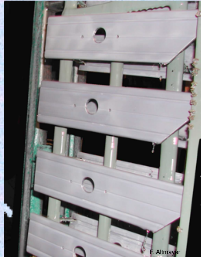
Zincated Aluminum Castings Non-uniform gray color indicates potential problem with zincate
